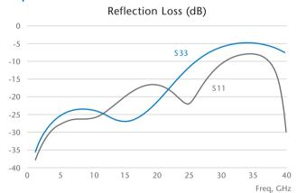
Further optimization of RF performance through better grounding can be achieved with additional wire bonding from pedestal to CuW block:
