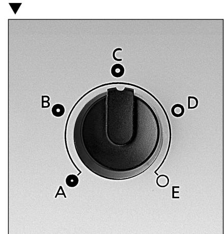
Position A gives the lowest brightness, and maximum brightness is achieved in position E (aperture completely open). Turning the adjustment knob from one retention point to the next approximately doubles or halves the light intensity respectively each time.
