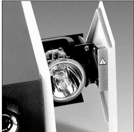
First of all switch off the light source. Open the lamp compartment (10) by pressing the button (11) and pull it out as far as the stop. Press down the two levers of the special socket and pull out the faulty lamp. The two levers must be pressed down again while inserting the new lamp. Push the lamp compartment in until it latches (audible locking sound). Switch the light source on.
