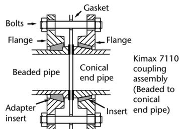
1. Disassemble coupling and remove inserts
