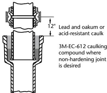
1. For line flexibility, place coupling within 12 inches of caulked joint.
