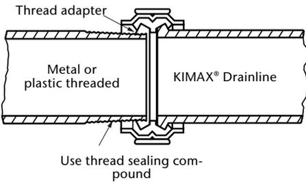
**KIMAX® Thread Adapter and Drainline Coupling**
