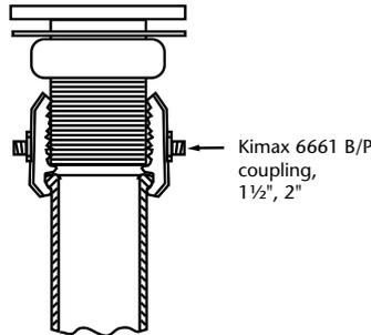
1. Snap coupling over beaded end of pipe or trap.
