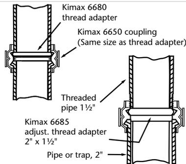
1. Screw thread adapter onto threaded pipe until it "bottoms". With adjustable adapter, screw into threaded pipe until desired height adjustment is reached.
