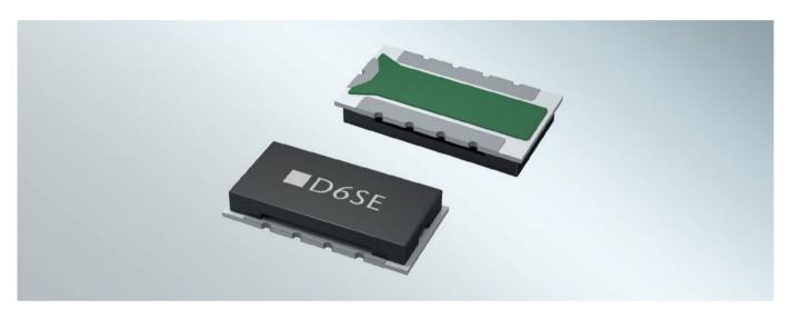
SCHOTT SEFUSE® D6S battery fuses are used in the secondary protection circuit of li-ion batteries to prevent dangerous circumstances of overcurrent and overcharging, and additionally help prevent fires caused by overheating. **D6SE series battery fuses** support rated currents of 30A, 45A and 60A and are well-suited for high-current applications, such as power tools and E-bikes.
