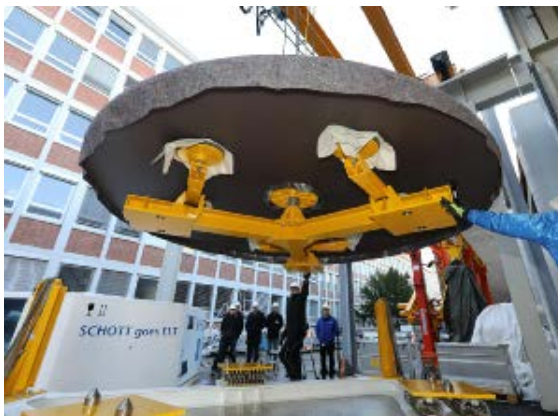
The secondary mirror support for the ELT is ten centimeters thin - and that with extreme curvature, 4.25 meters in diameter and weighing three tons. Photo: SCHOTT
