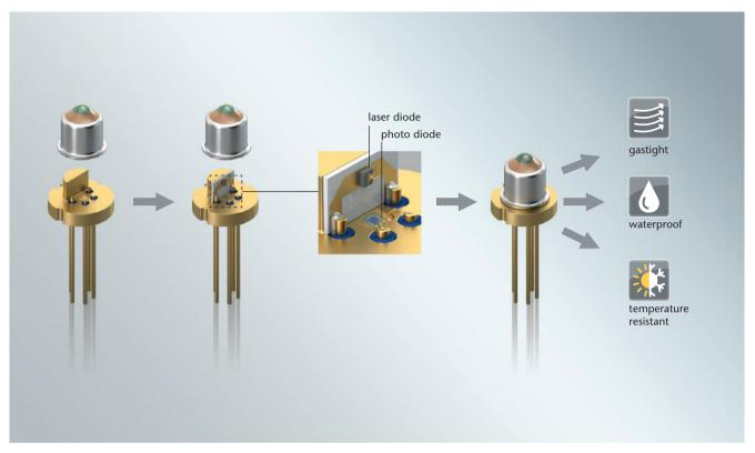
**TO cans – key components for hermetic protection:** Transistor outline headers and lenses are assembled to form a hermetically sealed "TO can" for reliable encapsulation, protecting sensitive semiconductor components from any adverse effects.
