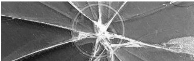
Figure 1: Close up picture of cracks in a ZERODUR® plate used to determine the bending strength experimentally.
