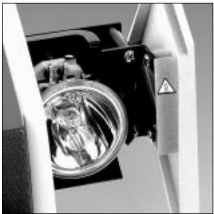
First of all switch off the light source. Open the lamp compartment (10) by pressing the button (11) and pull it out as far as the stop.
