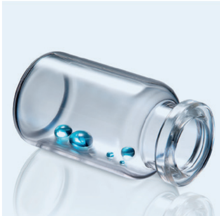
Silicization presence/absence and uniformity using colored water droplet test
