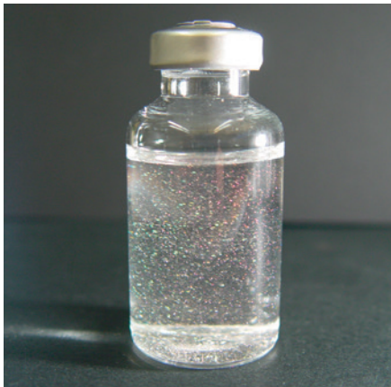
Flake-like particles by visual inspection
