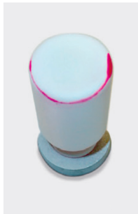
Dye penetration testing concerning glass container integrity
