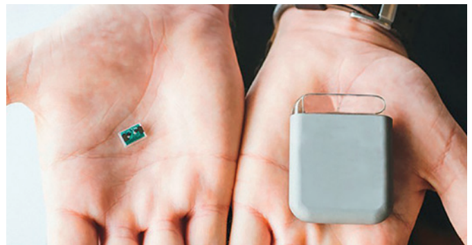
A side-by-side comparison showing a typical medical implant (right) and a SCHOTT Primoceler all-glass implant (left).
