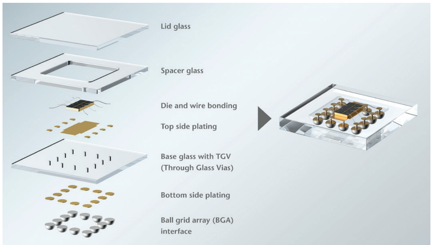
An explosion view diagram of a device encapsulated with Glass Micro Bonding.
