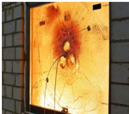
Test: Large fire test after gun shots
