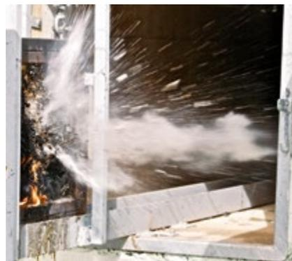
Test: Gun shots after small fire test
