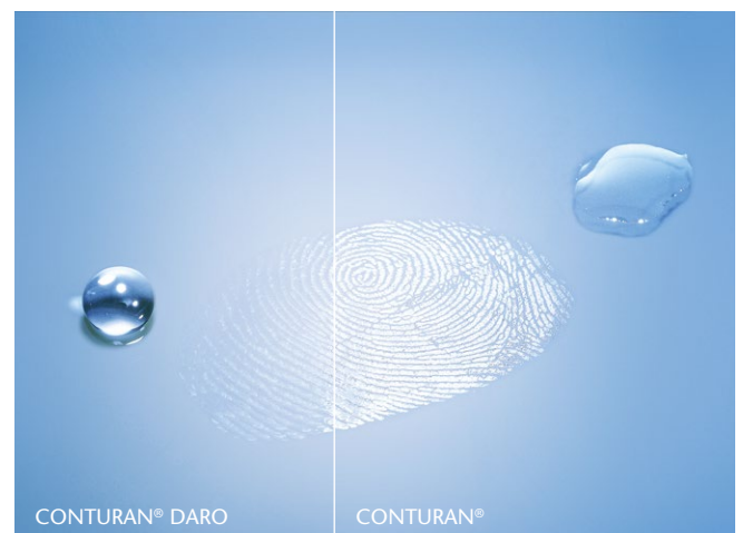
Fig. 33. Visual appearance of a finger print on CONTURAN® (right) and on CONTURAN® DARO (left)
