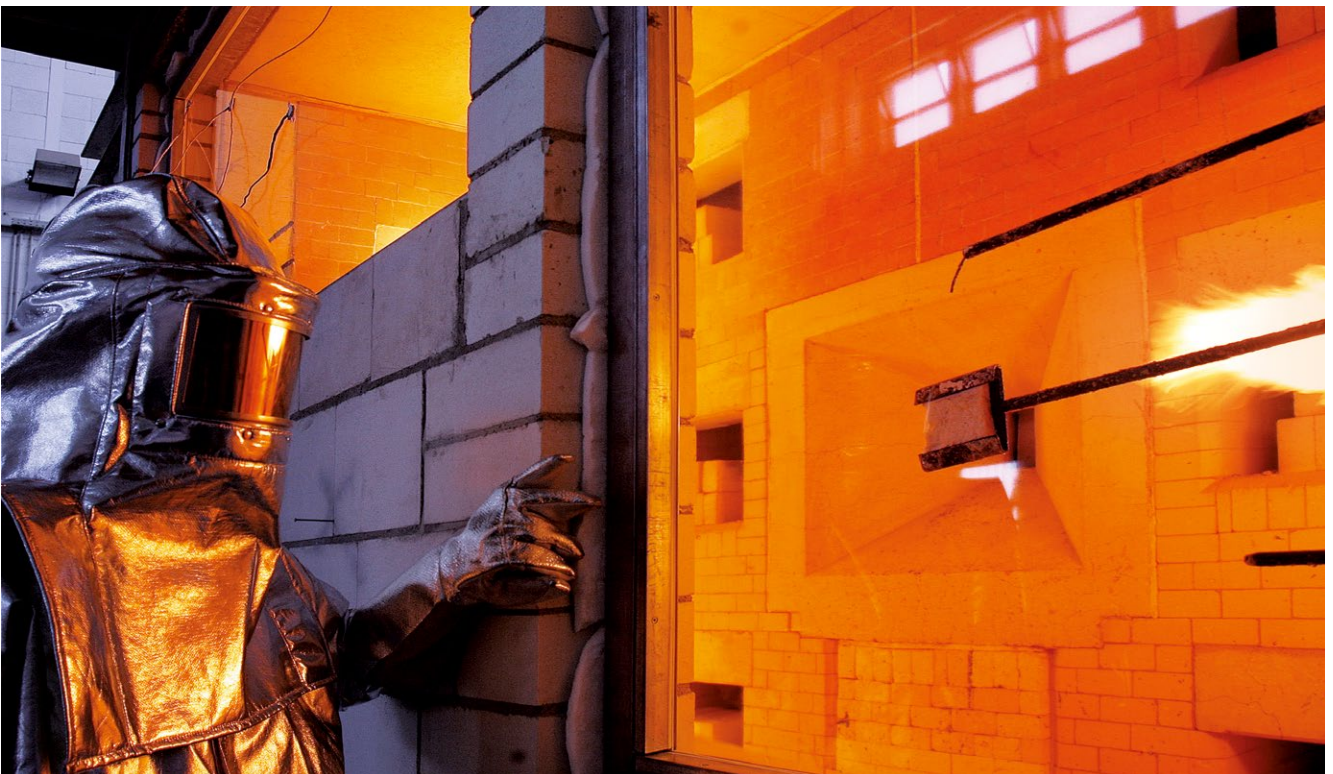
PYRAN® Platinum fire-rated glass-ceramic resists fire without fracturing.
