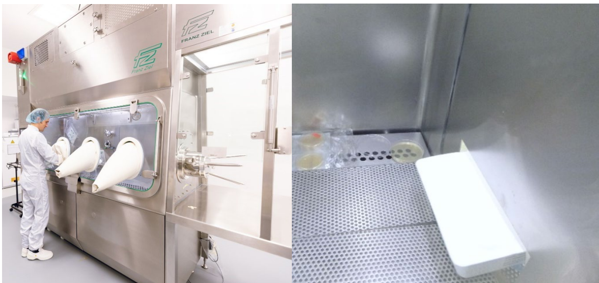
Figure 4: Picture of the isolator and UDAF clean bench. Transfer of the tub inside the isolator (Grade A).
