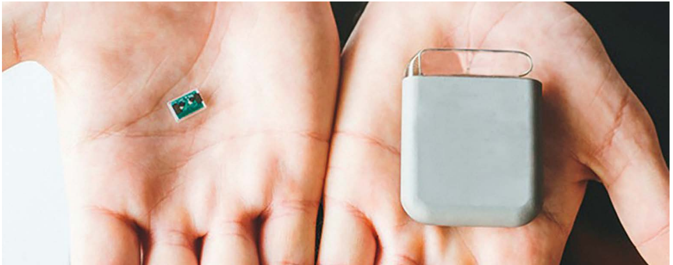
Side-by-side implants comparison showing a typical implant construction (right) versus the miniaturization properties of implants packaged with glass micro bonding technology (left). Image: SCHOTT
