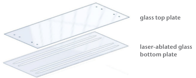
Two layer design with laser ablated channels
