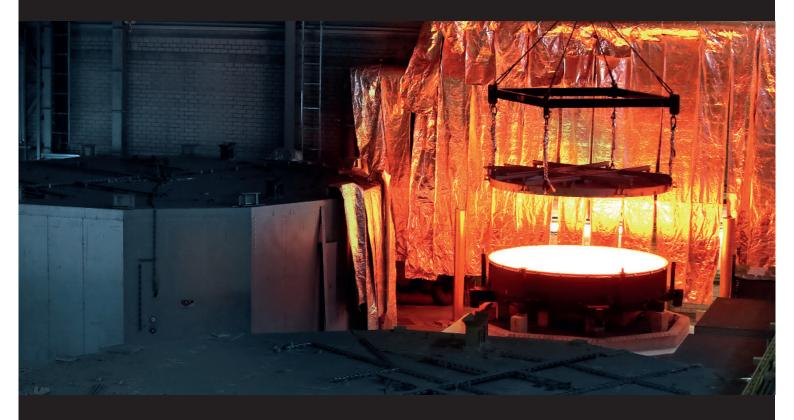
Production of the secondary mirror, with a diameter of 13.9 feet, recently got underway in mid-May of 2017. After grinding, the raw material is transformed into a strongly curved mirror – just ten centimeters or 3,94 inches thin.
