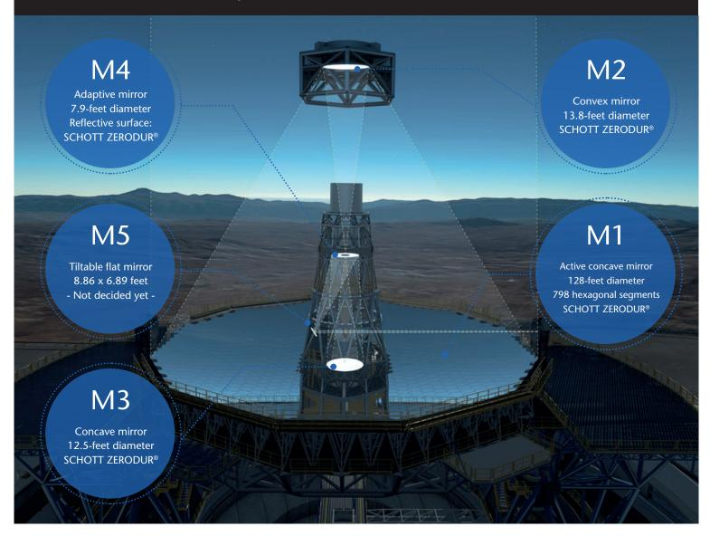
4 out of the 5 mirrors in the sophisticated optical system of the huge telescope are based on ZERODUR® glass-ceramic. Several hundred individual components come precisely together to work as a reliable team so that the light reaches where it is needed most – the ELT's cameras and spectrographs.
