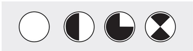
With the Ring Light Plus, you can rotate the segment setting step by step or set it to continuous rotation. Rotation mode increases the impression of three-dimensionality of structured objects, especially when viewed on the monitor.
