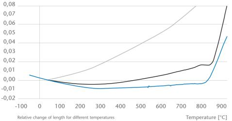
Thermal expansion in dependence on the temperature (for selected NEXTREMA® types)
