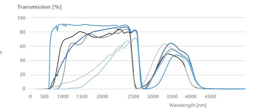
This graph is based on data from individual measurements. Deviations may result from manufacturing process. Typical transmission graph of different ceramization states with sample thickness of approximately 4 mm.
