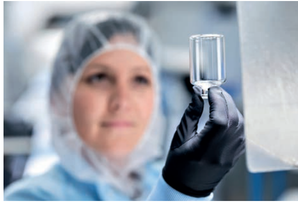
COVID-19 vaccine: In the future, vials made of borosilicate glass will be partially replaced by prefillable syringes made of polymer.
