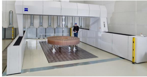
Large 3D CMM ZEISS MMZ-G since 2020
