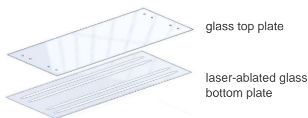
Two layer design with laser ablated channels
