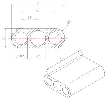
Geometry, Diameters, Lengths, Thickness, Number of holes to be defined according to customer request.
