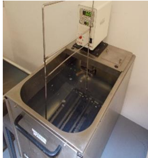
Figure 6: Temperature controlled cleaning baths work well for large batches of parts.
