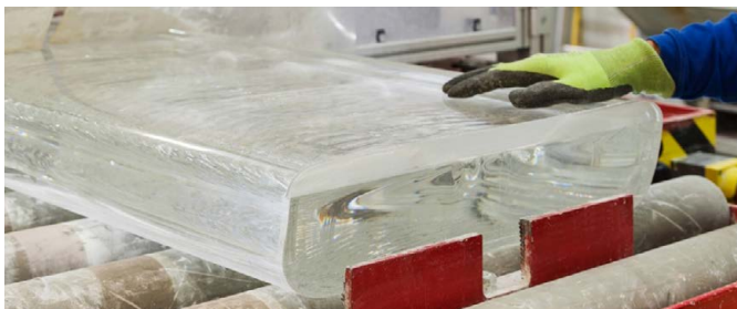
Fig. 17: SCHOTT N-BK7® strip glass with about 450 x 100 mm cross section
