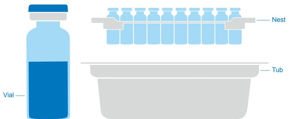
Figure 1: Components of a sterile ready-to-use packaging solution.
