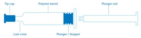
Figure 2: Polymer syringe system.
