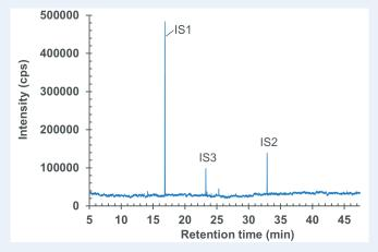
Figure 7: GC-MS chromatogram of polymer syringe barrel after extraction in water (pH 9.5).
