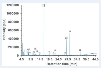
Figure 4: HS-GC-MS chromatogram of polymer syringe barrel component after incubation at 150 °C for 45 minutes.
