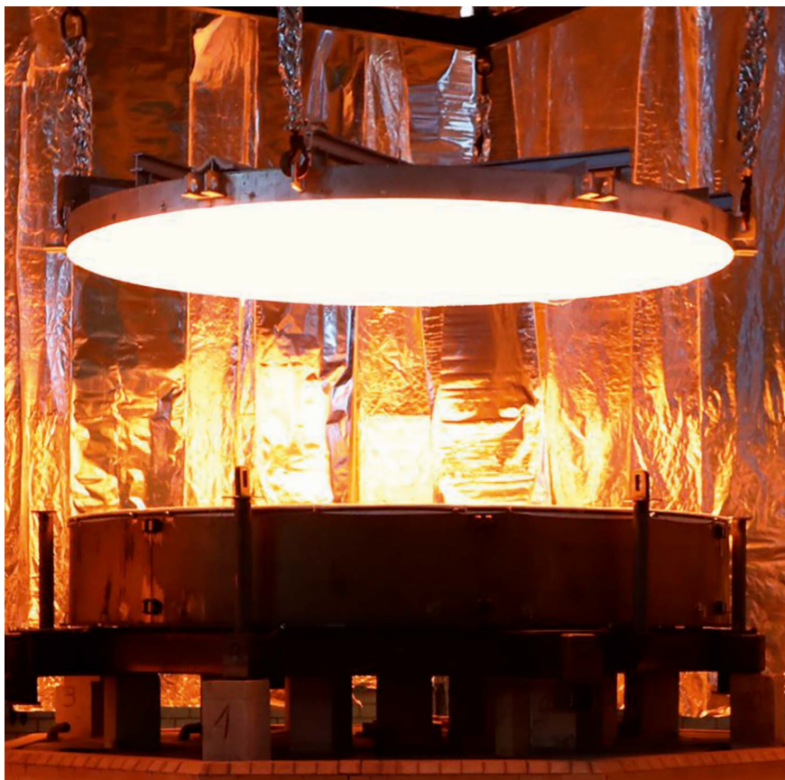
Annealing of a 4-m-class blank at SCHOTT AG
