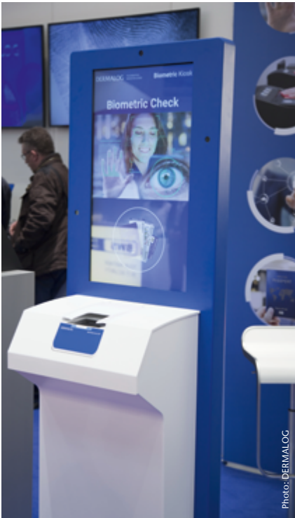
DERMALOG scanner at CeBIT 2017: on the same scan area it can read fingerprints as well as electronic passports.
