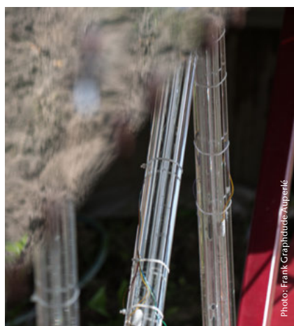
The bridge strut is made of DURAN® glass tubing.
