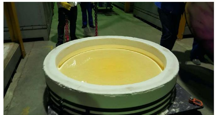
Fig. 16: Mould with a 1500 mm diameter SCHOTT N-BK7<sup>®</sup> casting.
