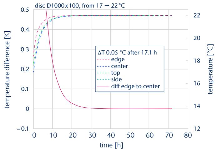
Fig. 15: Required temperature conditioning time for a 1000 mm diameter and 100 mm thick SCHOTT N-BK7<sup>®</sup> blank.
