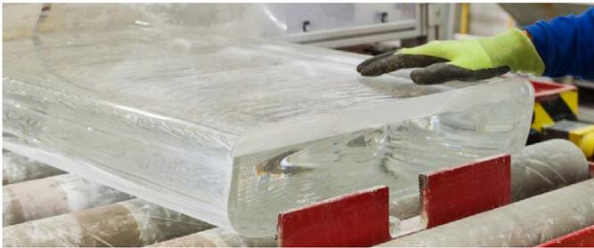
Fig. 17: SCHOTT N-BK7<sup>®</sup> strip glass with about 450 x 100 mm cross section
