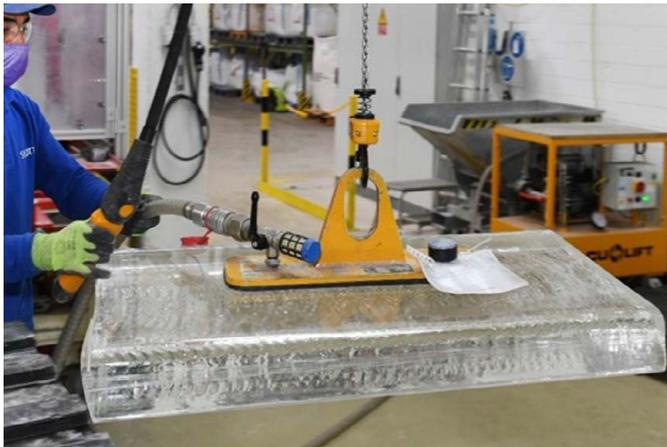
Fig. 22: 900 x 450 x 100 mm<sup>3</sup> continuously produced SCHOTT N-BK7® strip!
