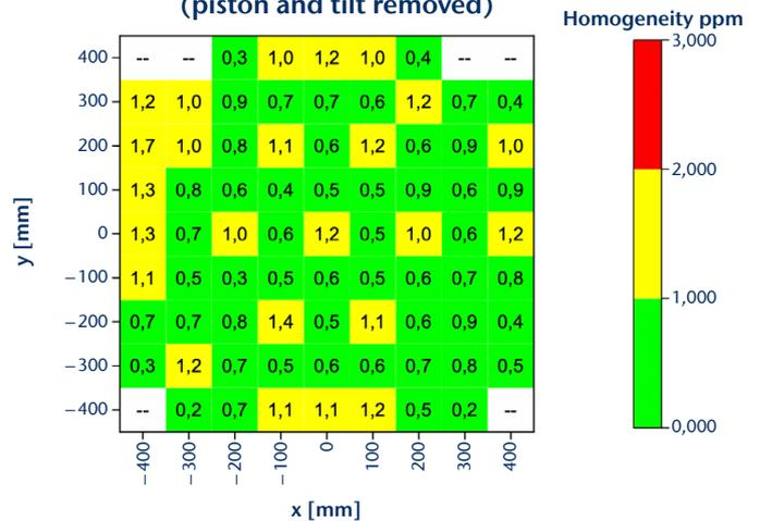
Fig. 20: The same blank yields H4 to H5 quality on all 100 x 100 mm sub-apertures (after piston and tilt subtraction)! The number in each square shows the peak-to-valley refractive index variation.
