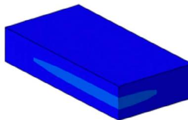
**Fig. 4:** Stress distribution in a rectangular SCHOTT N-BK7® blank for fast (left) and slow (right) annealing. Only a “quarter part” of a rectangular casting depicted (symmetry conditions are enabled to ease simulation).
