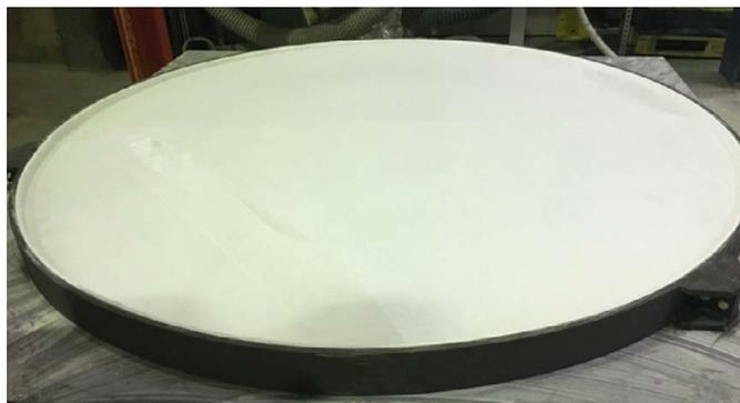
Fig. 18: 2200 mm diameter SCHOTT N-BK7<sup>®</sup> blank after slumping
