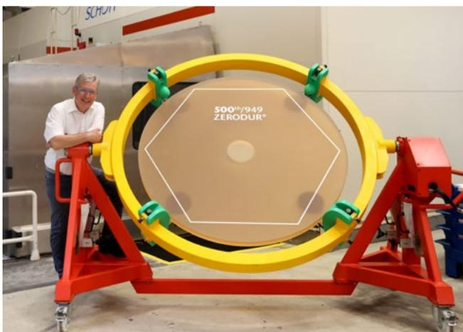
An important milestone along the way was reached in Mainz, Germany in July 2022. By completing the 500th mirror substrate for the ELT's M1 main mirror, the ZERODUR® team at Advanced Optics has successfully finished more than half of the mammoth task (see photo above). Due to its near-zero coefficient of expansion, the material is considered the gold standard for telescope mirror substrates.
