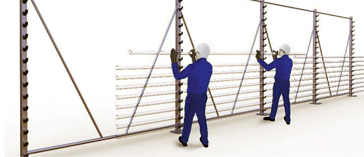
Handle glass with care: Have the tubes laid into their position by two people.
