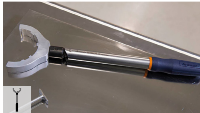
Torque wrench (Standard coupling: 40Nm, Slim coupling: 25 Nm)
