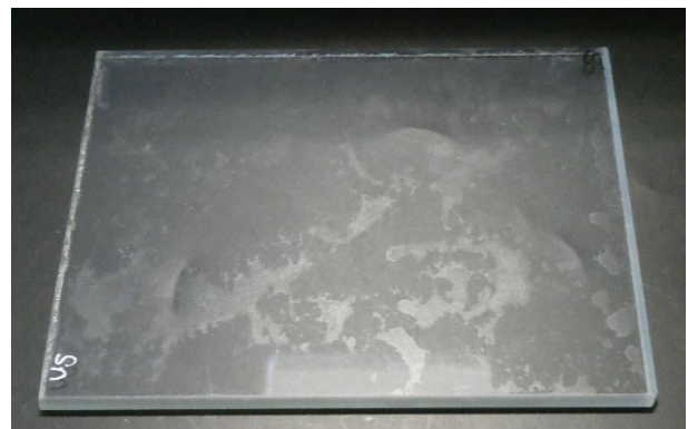
Figure 2: uncoated glass after the test: mould spots are clear visible
