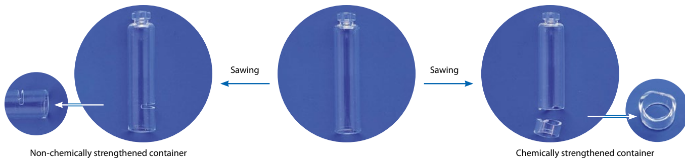
Figure 3 Sawing of a non-chemically strengthened (left) and chemically strengthened glass (right) glass container with a diamond-cutting disc
