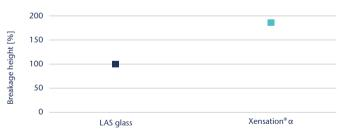
Mean values of dummy test series with 0.8 mm thickness, compared to LAS glass; results may vary depending on test set-up
