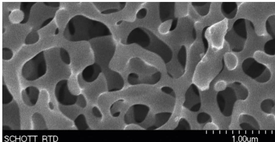
Cold field emission scanning electron microscope image of CoralPor® porous glass
