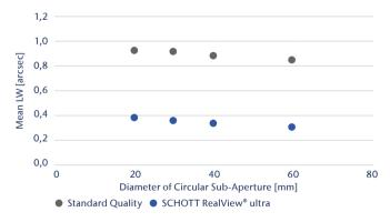
Mean local wedges for typical eyepiece-sized sub-apertures are cut by more than half for SCHOTT RealView® ultra compared to standard market quality.
