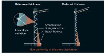
Propagation of a light beam through a waveguide. The number of bounces increases with reduced substrate thickness. Wedge causes systematic deviation of the light beam. Local deflections can occur due to local slope.
