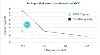
Vials produced with a standard converting process served as benchmark.
