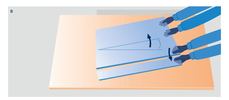
Always make these relief cuts continuously up to the glass edge! First break the relief cuts parallel to the drawing direction, then crosswise to the drawing direction. The long and narrow strips in particular are easier to break if a second person assists with breaking by lifting the sheet approx. 5 – 10 cm from the cutting table and the cutter breaks off the narrow strip (graphic B).
