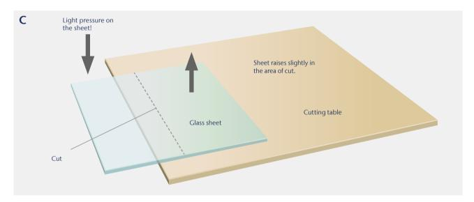
Where the glass format and cutting plan allow, breaking the glass "over the edge" will provide a better result than breaking on the cutting table. Please proceed as follows: Turn the flat glass with the cut parallel to the edge of the table (graphic C). The distance between the cut and the edge of the table depends on the thickness of the glass and the size of the cut. Let the protruding part of the flat glass hang over the edge of the table. Never let go of the pane!
