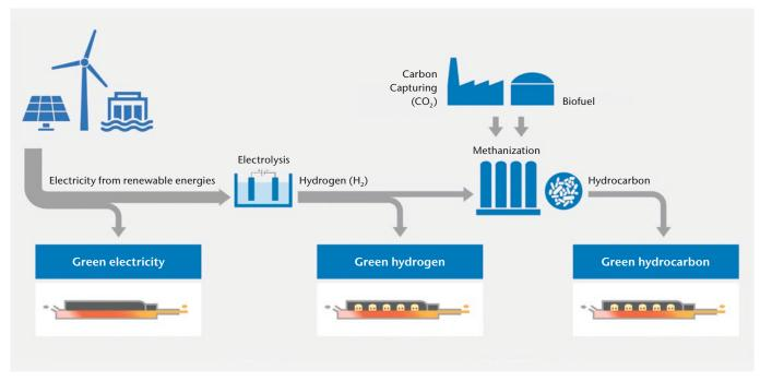
SCHOTT is pursuing three approaches to technological change. Electricity from renewable energy sources forms the starting point for them all. The most efficient is the direct use of green electricity. In comparison, the overall efficiency of hydrogen and hydrocarbons decreases because some of the electrical energy originally present is lost during their production.
