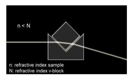
At SCHOTT, we custom built a V-block refractometer that not only acquires measurements with higher accuracy than commercial systems but also makes the process more efficient by incorporating automation.
