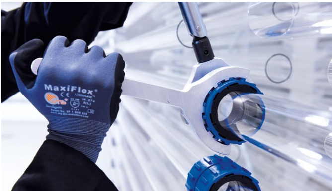
7 The jaw wrench should be placed accordingly on the right side of the coupling.
