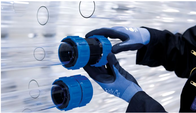
5 The other glass tube can now be pushed into the other end of the cage and both tubes are now in their final position. Push the nuts over the cage.
