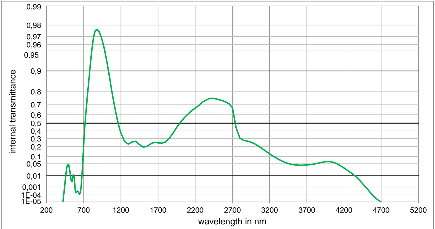
Internal transmittance \tau_i at reference thickness The internal transmittance values, tabulated and graphically represented, are reference values only
