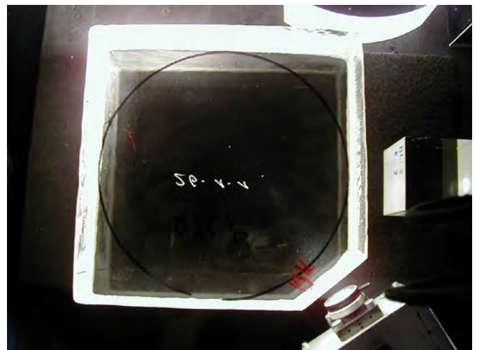
Fig. 1: Optical glass block with a small amount of bubbles.
