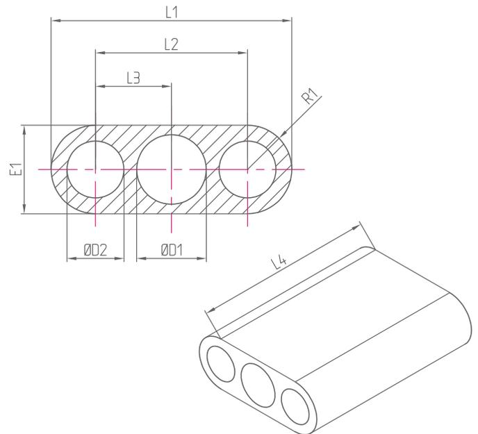
Geometry, Diameters, Lengths, Thickness, Number of holes to be defined according to customer request.
