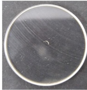
Uncoated sample shows clearly scratch marks over the whole surface
