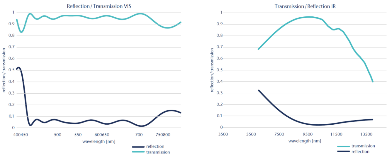
Figure 2: Transmission and reflection curves of a scratch resistant 2-band AR coating (VIS+LWIR).
