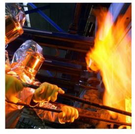
The goal of climate neutrality is a great challenge for a specialty glass manufacturer like SCHOTT: Specialty glasses and glass-ceramics are melted in large melting tanks at temperatures of up to 1,700 degrees Celsius. A lot of energy is required for glass melting and further processing.
