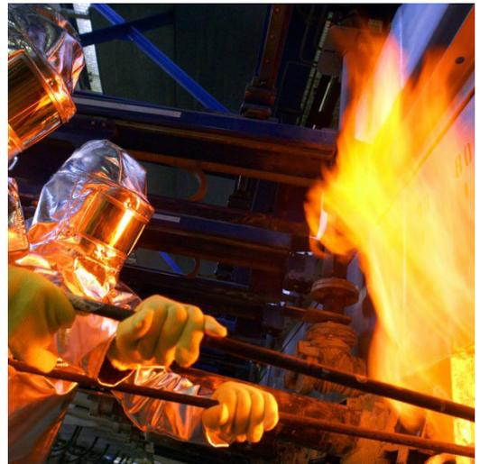
The goal of climate neutrality is a great challenge for a specialty glass manufacturer like SCHOTT: Specialty glasses and glass-ceramics are melted in large melting tanks at temperatures of up to 1,700 degrees Celsius. A lot of energy is required for glass melting and further processing.
