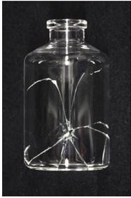
Macroscopic fracture patterns (Figure 2) are the crack and crack branching patterns, visible by eye or with low magnification, which develop due to the momentary mechanical stress
