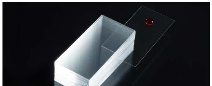
D 263<sup>®</sup> M cover glass, produced with the SCHOTT proprietary Down-Draw process, has a chemical composition that ensures valid and reliable research results. This is due to low autofluorescence and high chemical resistance, as well as a refractive index finely tuned to microscopy use. With standard thicknesses from 0.1 mm to 0.21 mm, it's also available from stock in a wide variety of easy-to-cut sheet sizes.
